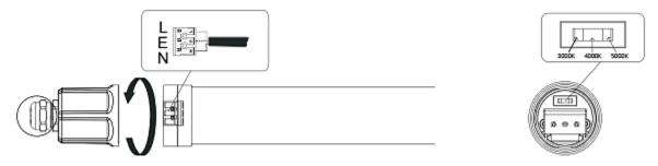
Twist the end cap and connect the cable.
